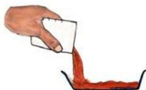
**Step 5** Mix sample with the solution by tilting the tray for 10 to 15 seconds until it turns dark-violet in colour.
